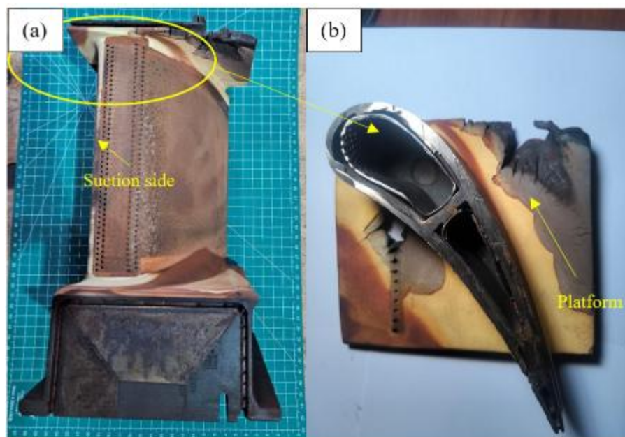
Figure 1. (a) General view of first-stage vane consist of damage in platform endwall corner, (b) Macrography examination of damage
